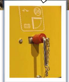
The combine harvester is equipped with either mechanical or electrical master switch.
